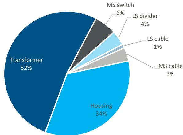
Figure 2 -CO<sub>2</sub>-emission installed transformers
