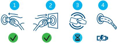
Figure 2.4: Starting the charging process with user authorization / charge card. Symbols shown on the user interface
