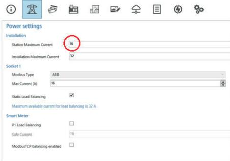
5. Enter the maximum value of the (grid) connection at the *Installation-MaxCurrent* bar
