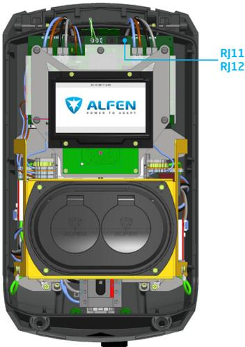
Image 3: Location RJ11/RJ12 connector on CTL920 controller board
