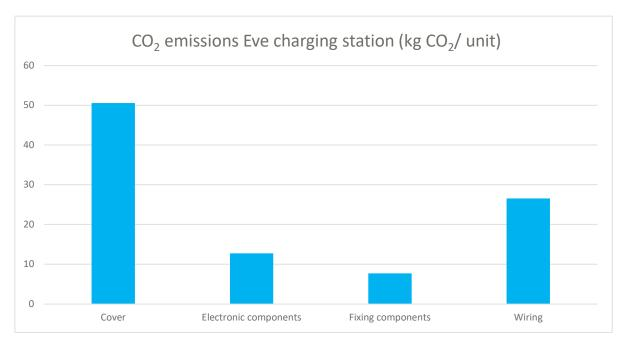
Figure 3 - CO<sub>2</sub> emissions main components Eve Charging station
