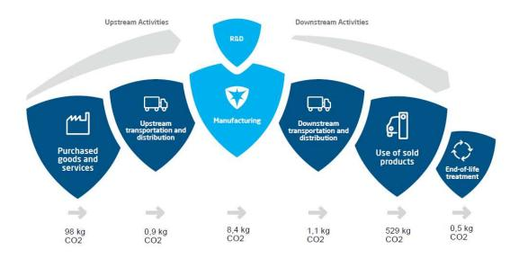
Figure 6 - Carbon footprint Alfen Eve charging station
