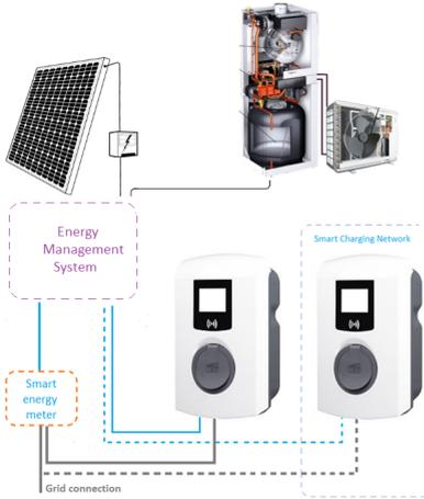
Figure 5.5: Active Load Balancing with Energy Management System and PV and heatpump
