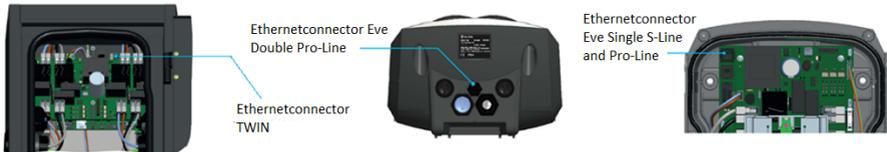
Figure 5.15: Ethernet connector locations
