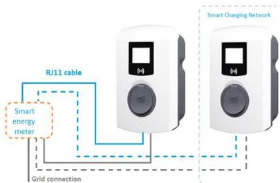
Figure 5.2: Active Load Balancing with energy meter (P1 part)
