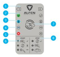
Figure 2.8: Display of Twin 5 with LED's (left socket active in this illustration)
