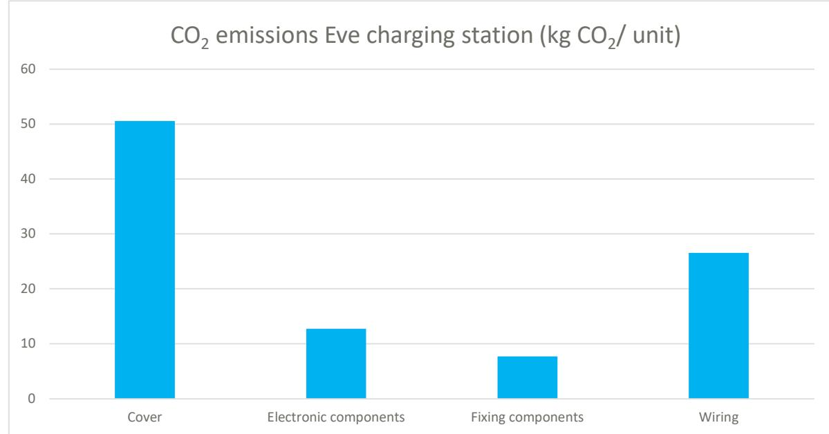
Figure 3 - CO<sub>2</sub> emissions main components Eve Charging station
