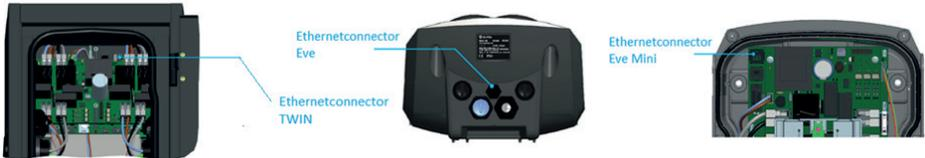
Figure 4: Location Ethernet connector charging stations
